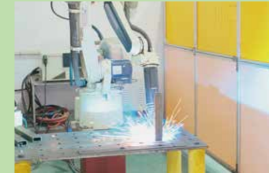
Robot welding operation
